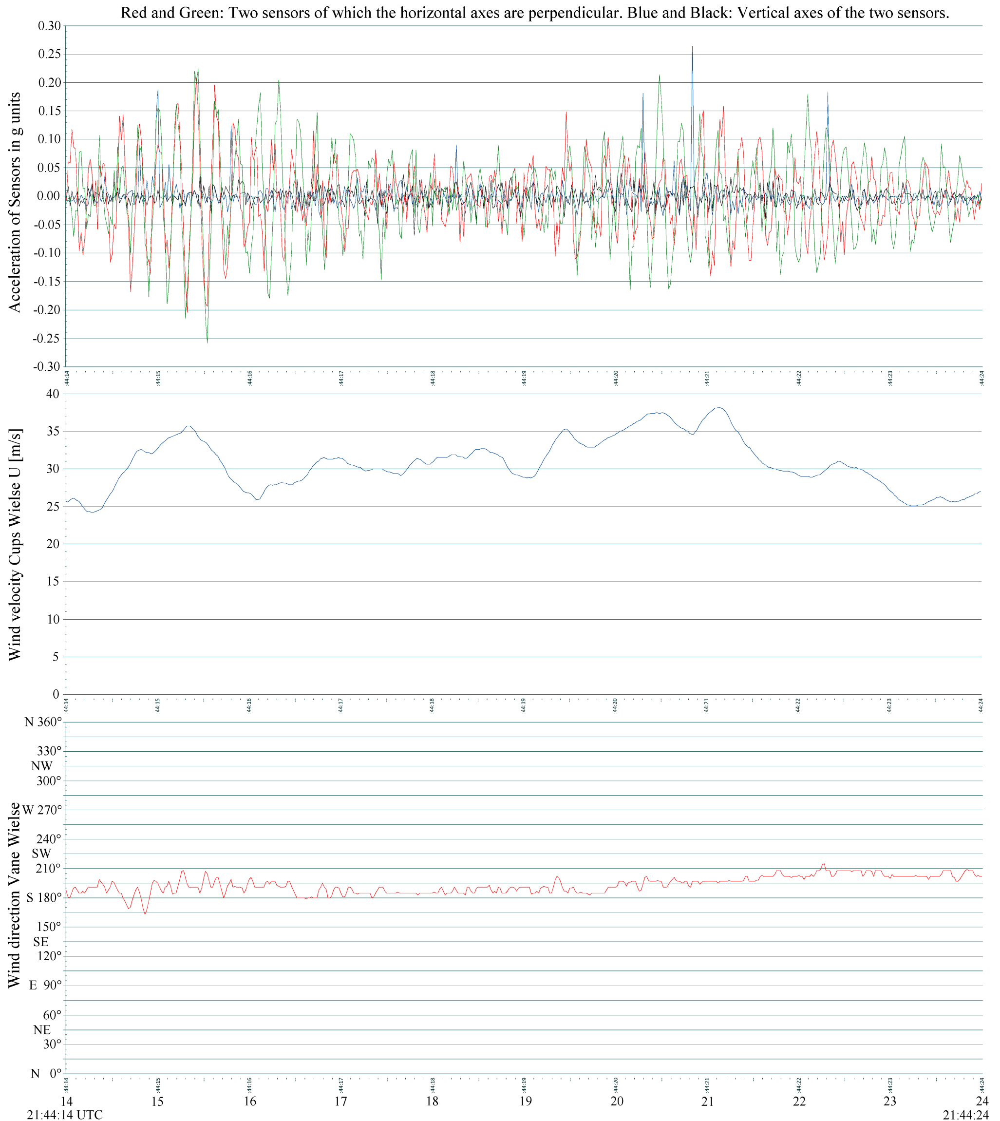
Figure 10. The acceleration measurements on the Transmitter tower during the 10 seconds with the strongest gusts UTC time 21:44:14 till 21:44:24, local time 23:44:14 till 23:44:24.
