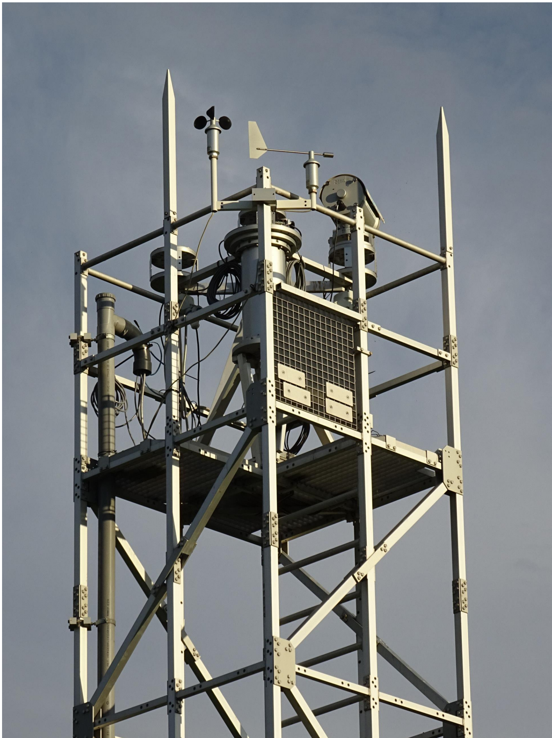
Figure 3. Top of the first tower with also the additional instruments installed. The LAS transmitter is seen from the backside pointed with his front lens towards the LAS Receiver. The cups anemometer and vane are seen on the nearest corner point of the tower top. The many visible cables are from the highly sensitive acceleration sensors. A second peak is mounted for lightning protection of the additional instruments.
