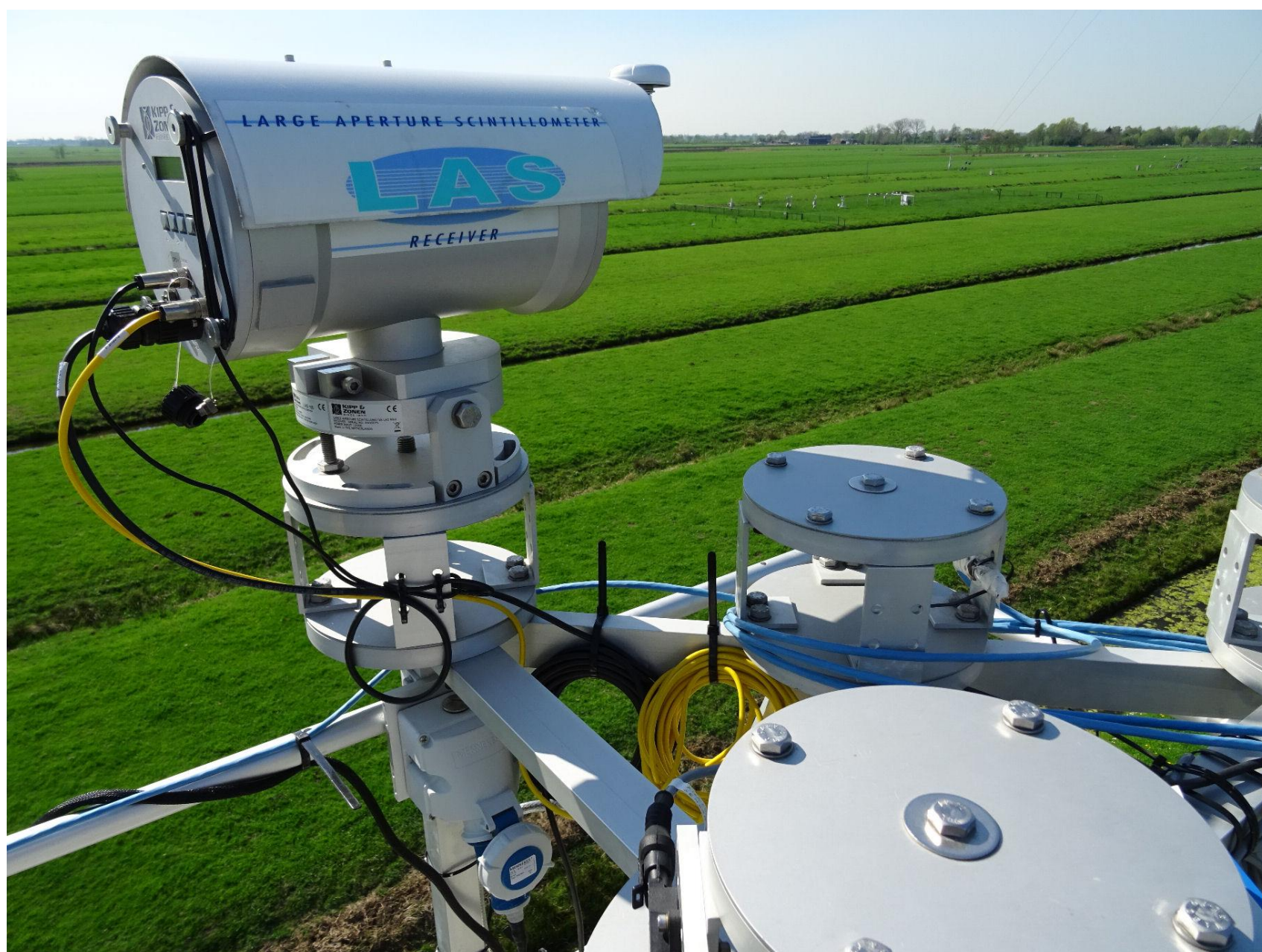
Figure 6. Close-up of the LAS Receiver and the four base platforms for instruments on the second tower.
