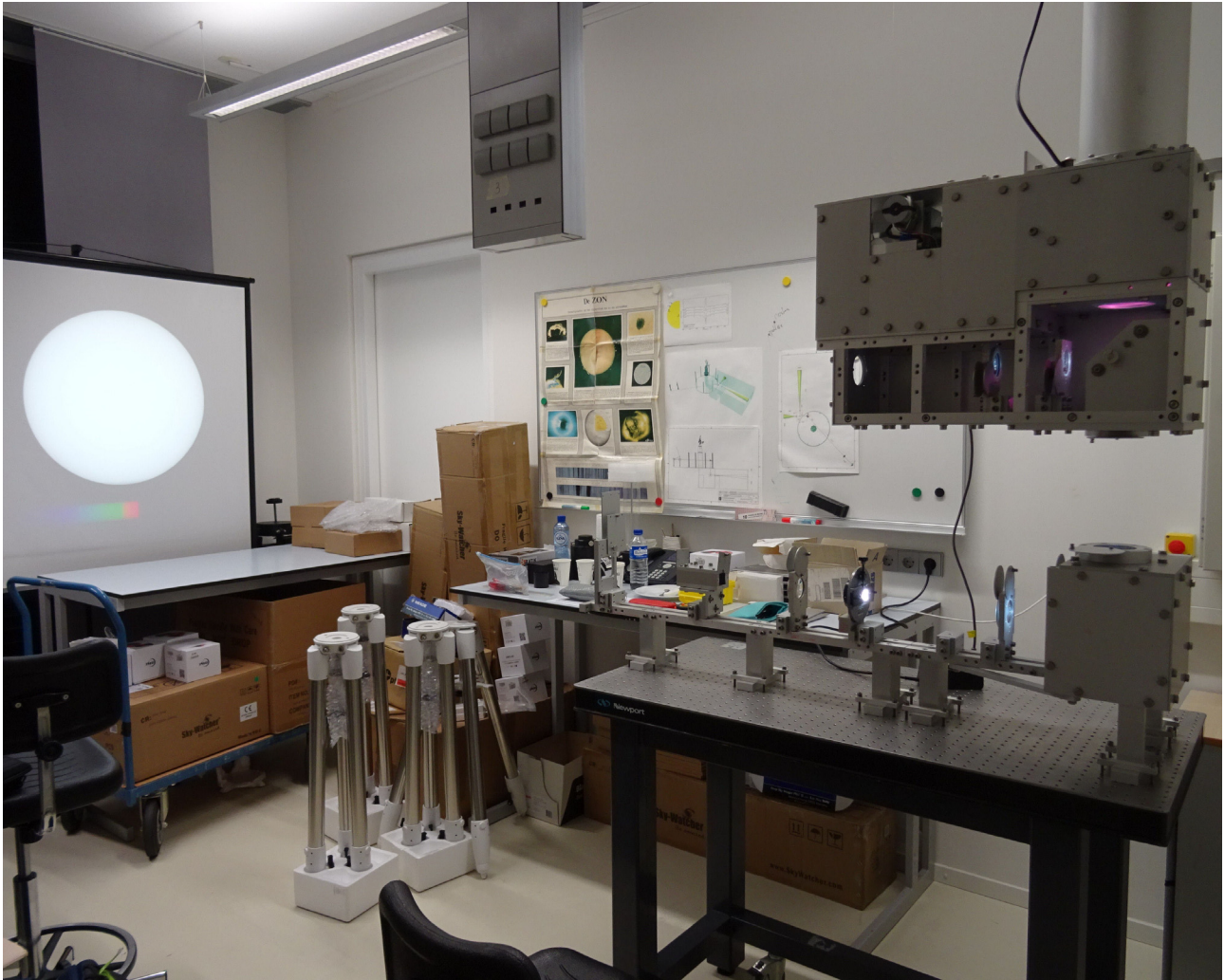
Figure 4. The setup in the Heliostat room from end of downward dome tube to projection screen. The lights in the room are on to show the instrumental setup.
