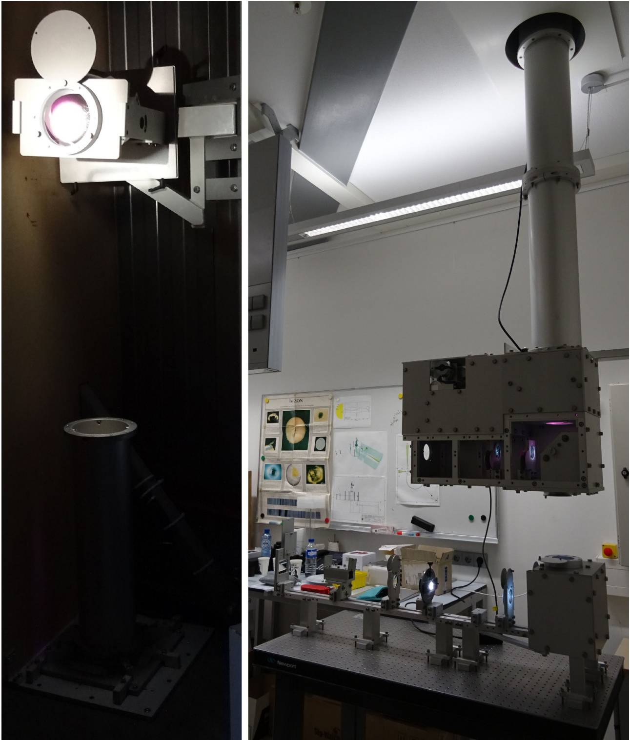
Figure 3. The downward light path from dome to Heliostat room.
