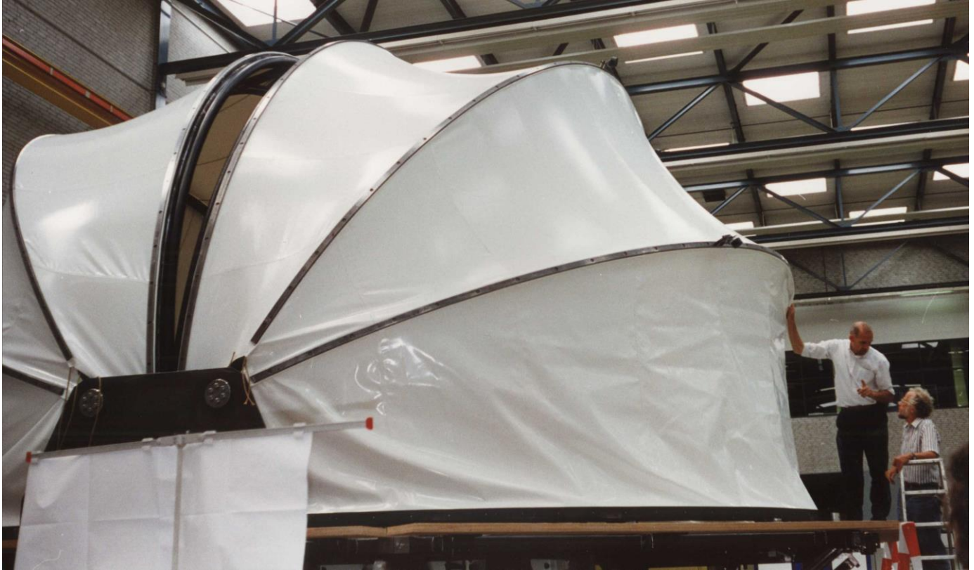
Figure 15. Test assembly of the DOT dome in the workshop of Delft University of Technology.
