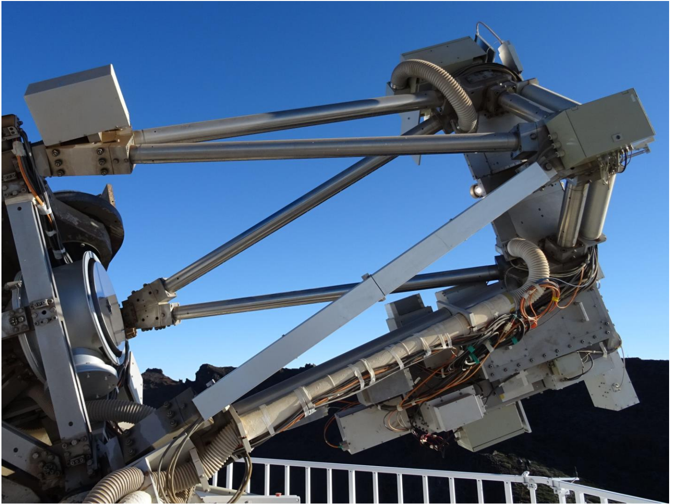
Figure 19. Observing DOT in the later afternoon. Left the primary mirror of 45cm diameter and 1997mm focal length. The primary image of the sun with diameter of 18mm diameter is visible as a very bright spot on the diaphragm plate, which selects a small part of the solar image, which goes through a hole in the diaphragm plate to the secondary optics.
