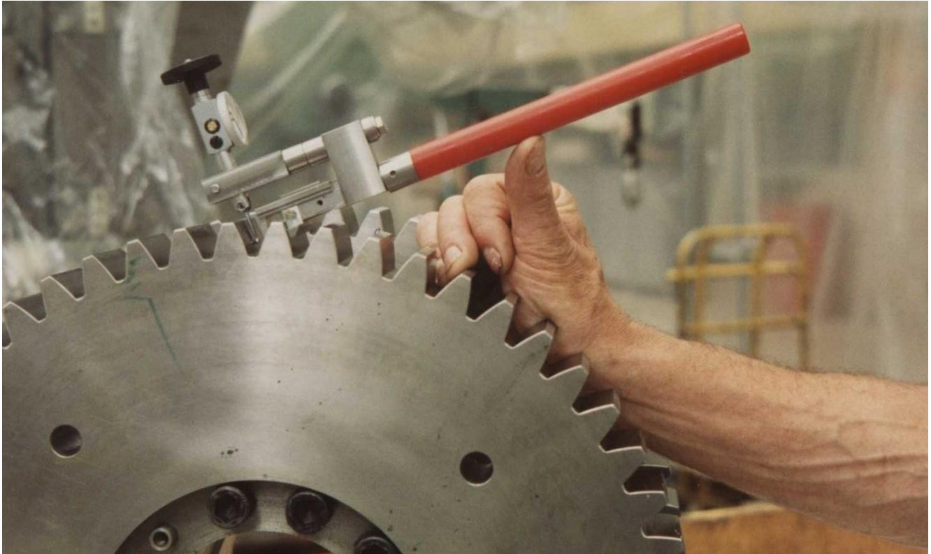
Figure 24. Side view showing how the pitch measuring instrument works. A small block is pressed against a tooth – the height is adjustable with a second small block behind the tooth. The instrument is so-to-say lying on a tooth. The gauge pin is behind the second block and hits the next tooth. The red plastic handle is moved up and down and the maximum push-in of the gauge corresponds to the minimum distance, i.e. the pitch. The person moving up and down the handle can read the \mu\text{m} gauge as Figure 25 is showing.
