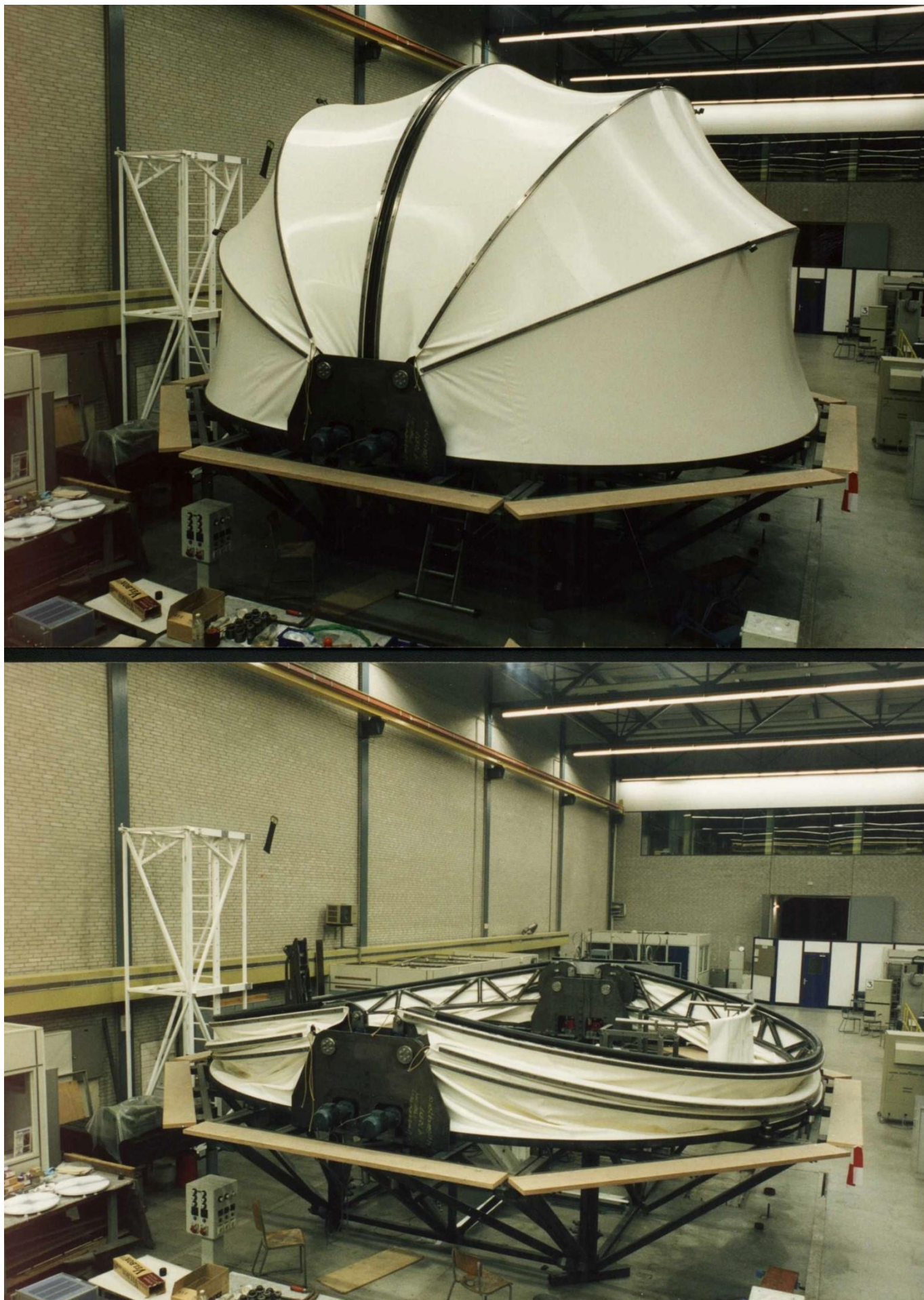
Figure 15a. In the workshop of Delft University of Technology the test assembly of the open platform for the DOT with the open foldable dome, closed in the top image and open in the bottom image.
